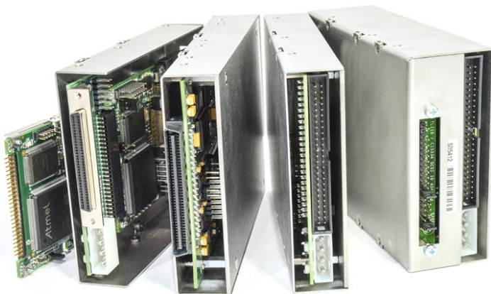
50-pin, 68-pin and 80-pin variants supporting 2.5 inch, 3.5 inch or larger 5.25 inch form factors
