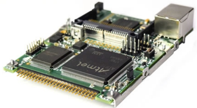
2.5 inch Hot Standby Drive variant. Single Slot CF (media) available
